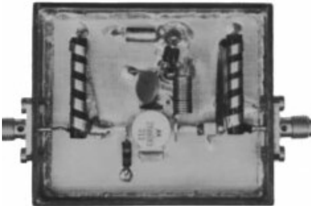
118 – 136 MHz Amplifier (see Figure 37) Before Coil Adjustment
